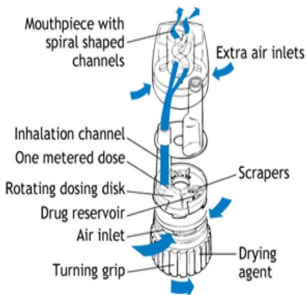
Figure 6: Schematic presentation of Turbuhaler®
