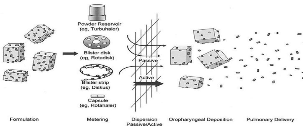
Figure 1. Principle of dry powder inhaler design.
