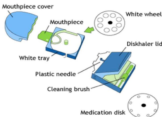
Figure 4: Schematic presentation of the Diskhaler®
