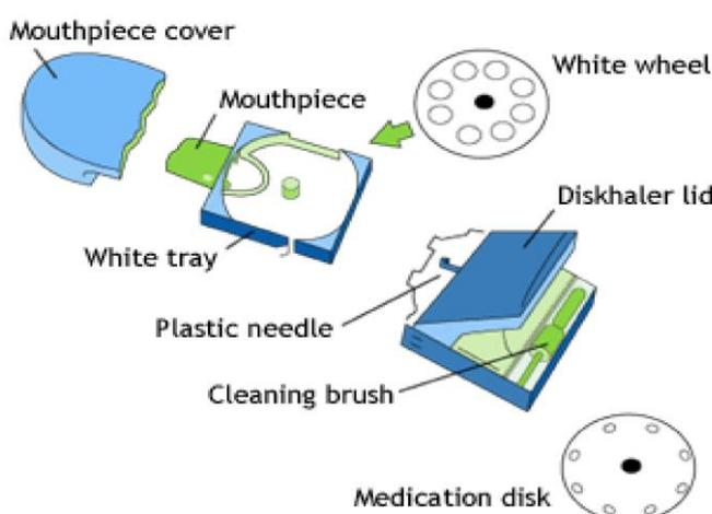
Figure 4: Schematic presentation of the Diskhaler®
