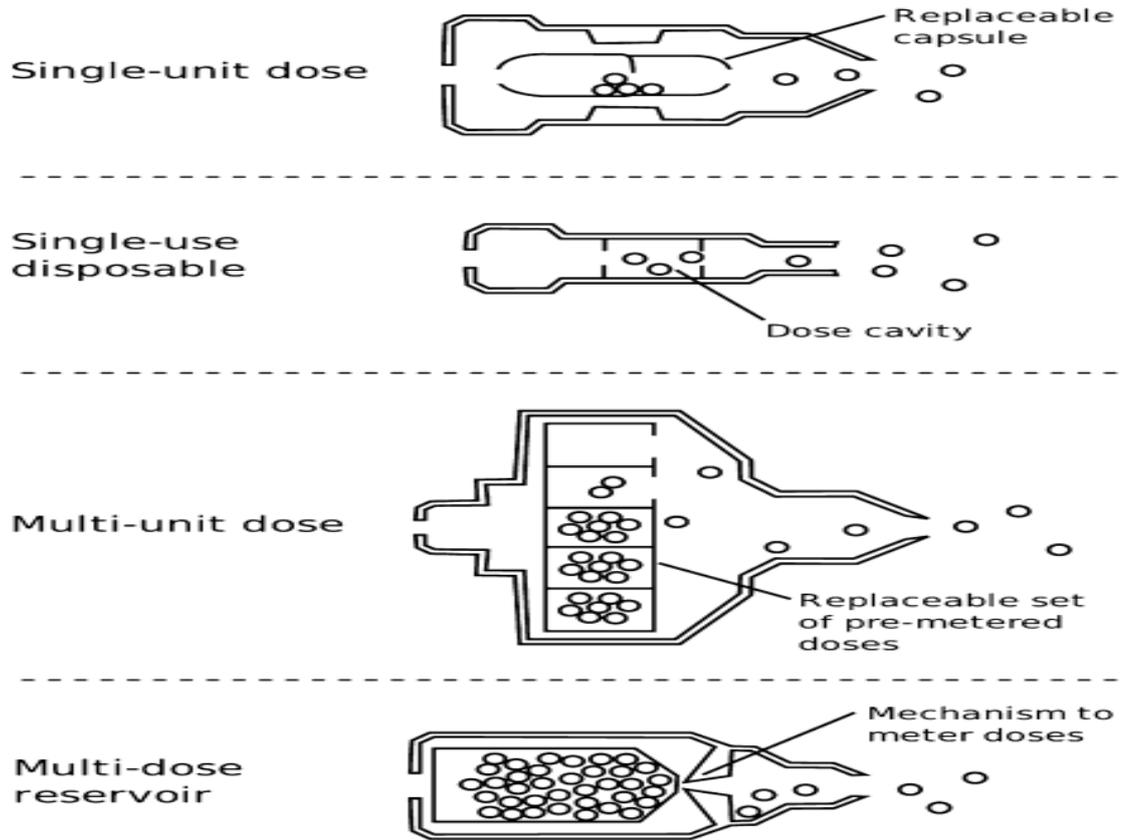
Figure 2: Illustration of four dose design options available for dry powder inhalers. [15]
